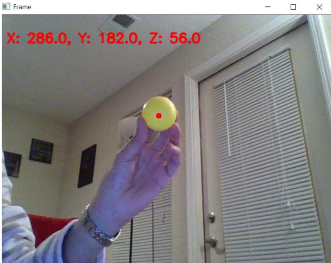
Figure 17: The resulting implementation of center finding using openCV
