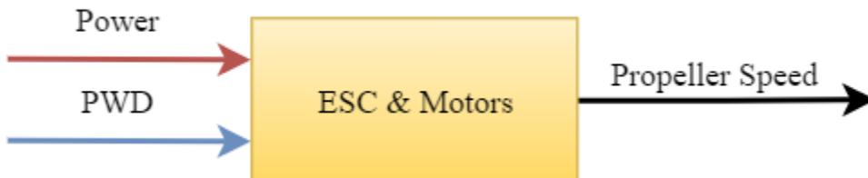
Figure 03 - ESC & Motors Level 0 Block Diagram [CC]
