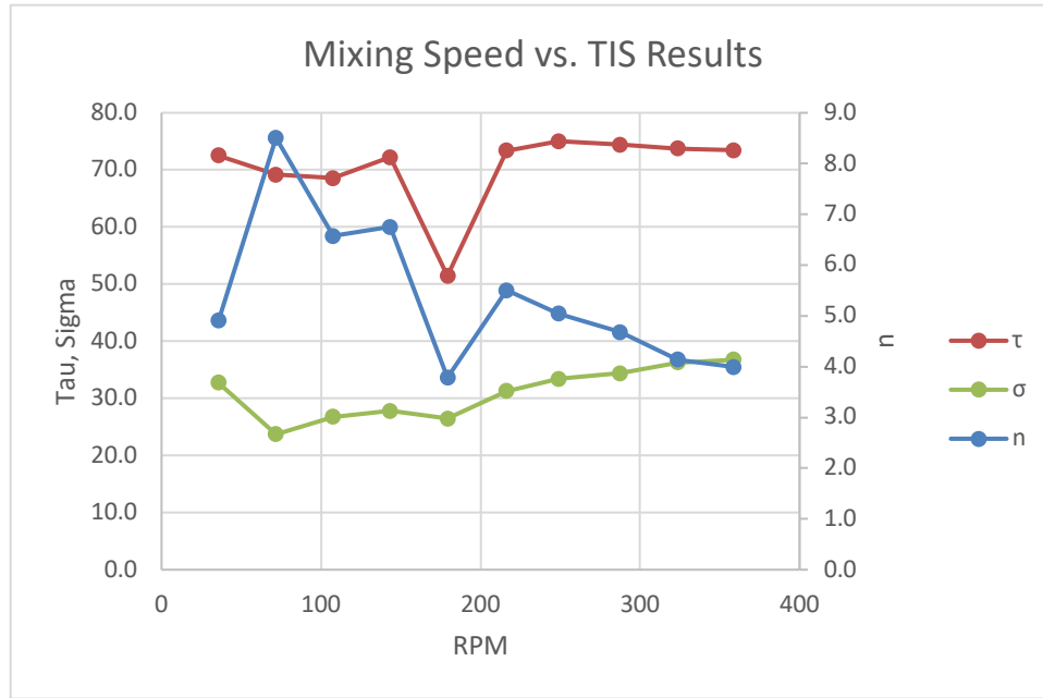
Figure 22: Comparison of tanks-in-series model parameters, \tau_m , \sigma , and n , vs. mixing speed for the second round of mixing speed tests. The second round of testing produced clearer trends in model parameters vs. mixing speed, and less overall scatter between the data. \tau_m and \sigma increased slightly as mixing speed increased, while n decreased significantly as mixing speed increased. This supports the conclusion drawn from the RTD curves in Figure 20 that the behavior moves farther from plug flow as mixing speed increases.
