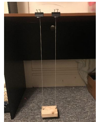
Figure 8: Setup to determine the moment of inertia about the y-axis of the wooden block
