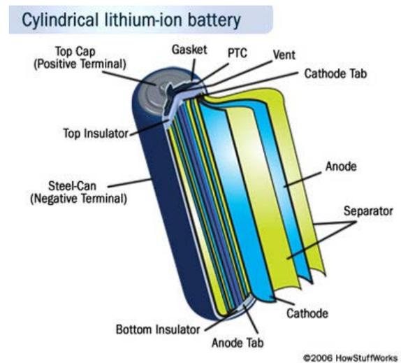
Figure 3: Cylindrical Lithium-Ion Battery [10]
