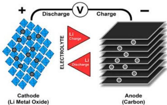
Figure 2: Depiction of Ion transport occurring in Lithium-ion batteries [1]
