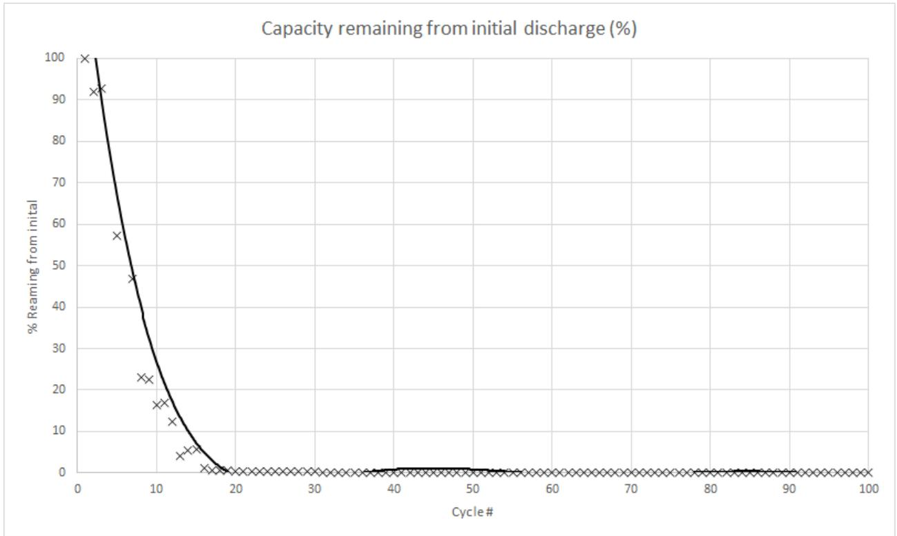
Figure 7: Composition 3 cycle testing showing degradation of capacity
