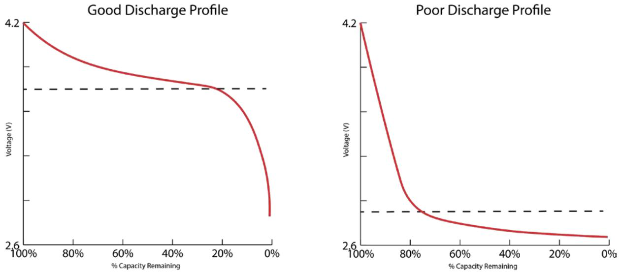
Figure 4: Battery discharge curves
