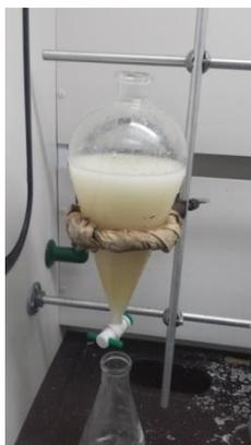
**Figure 7:** Example of the emulsion that forms during DI water/brine washes that can take hours or days to separate.
