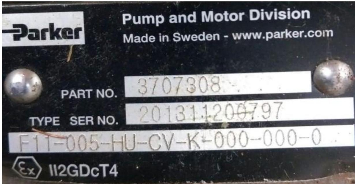
*Figure 1: Pump/Motor Part Number*
