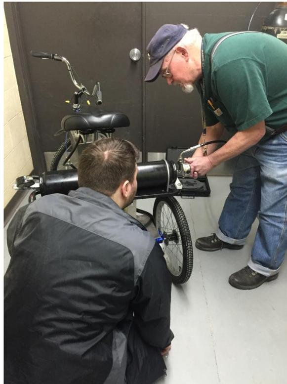
**Figure 3: Pre-charge accumulator**
