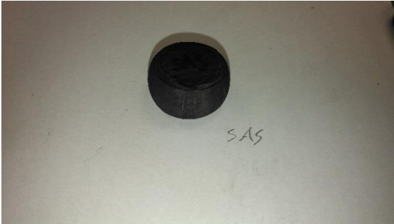
Figure C11. Compression Slug SAS sample after destructive testing. A few minor hairline cracks forming on the perimeter of the sample
