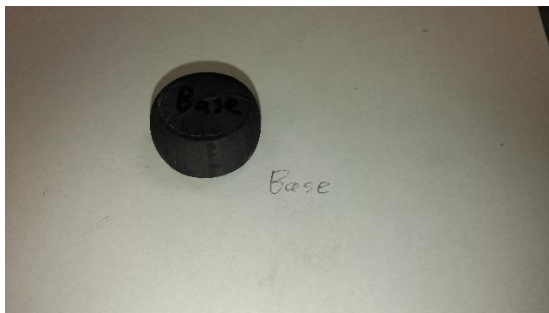
Figure C10. Compression Slug Base sample after destructive testing.
