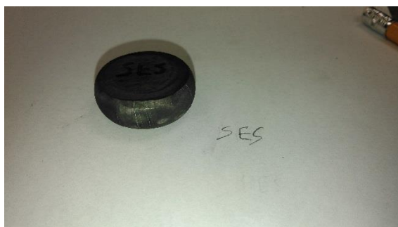
Figure C15. Compression Slug SES sample after destructive testing. Multiple hairline fractures began to propagate on the sides of the sample.
