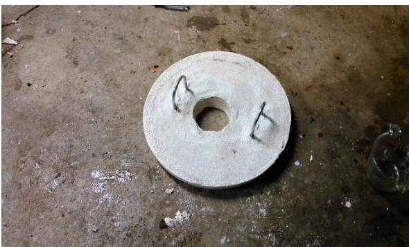
Figure B4. The lid of the forge with the vent hole drilled in the middle and the two U-Bolts on either side of the vent to accommodate the removal of the lid during operation. Unfortunately, due to operator error, the lid shown in this image cracked in half and was later discarded.
