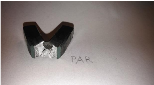
Figure C7. Charpy Impact PAR sample after destructive testing. The sample did not completely break, both sides are still connected. Very ductile break.
