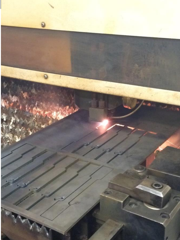
Figure D2. The tensile coupons being laser cut.
