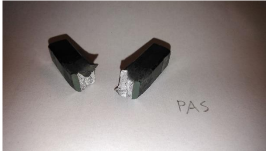
Figure C6. Charpy Impact PAS sample after destructive testing. Ductile break with both sides separating.
