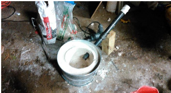
Figure B3. The forge with the steel air supply tube supported by a wood block checking the seal of the pipe to the forge walls.
