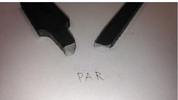
Figure C23. Tension Coupon PAR sample after destructive testing.
