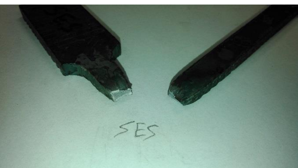
Figure C24. Tension Coupon SES sample after destructive testing.
