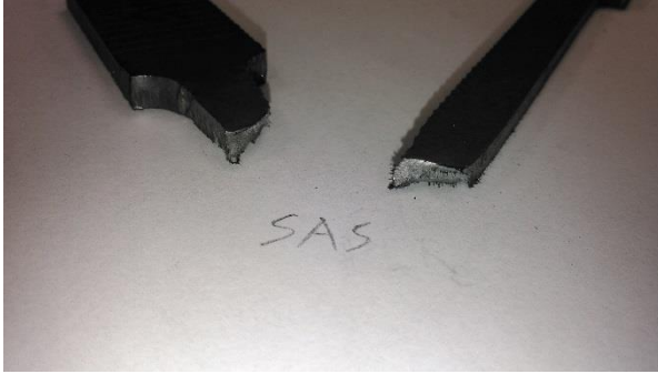
Figure C20. Tension Coupon SAS sample after destructive testing.
