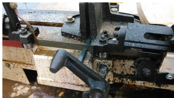
Figure D3. The Charpy impact samples being cut.
