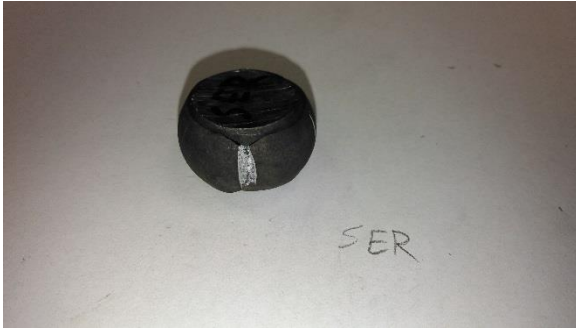
Figure C16. Compression Slug SER sample after destructive testing. Note the large fracture on the front face of the sample. Smaller fractures began to develop on the other sides of the sample as well.
