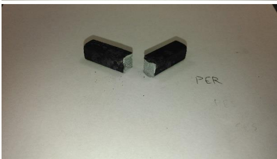
Figure C9. Charpy Impact PER sample after destructive testing. Nearly a perfect shear break. Shows signs of extreme brittleness.
