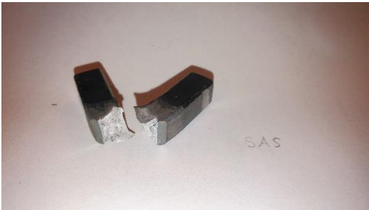
Figure C2. Charpy Impact SAS sample after destructive testing. Ductile break with both sides separating.
