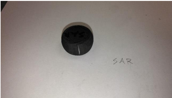
Figure C12. Compression Slug SAR sample after destructive testing. Note the fracture beginning to propagate on the one side.
