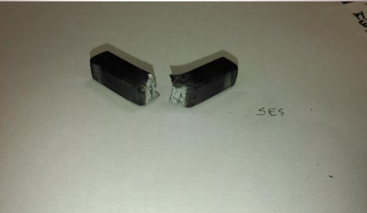
Figure C4. Charpy Impact SES sample after destructive testing. Ductile break with both sides separating.
