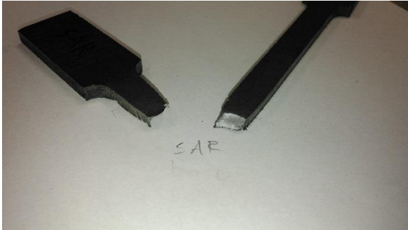
Figure C21. Tension Coupon SAR sample after destructive testing.
