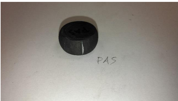
Figure C13. Compression Slug PAS sample after destructive testing. Note the fracture beginning to propagate on the one side. A hairline fracture is beginning to propagate to the left of the main fracture as well.
