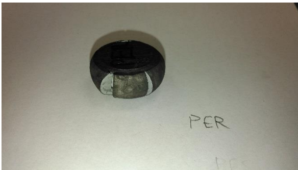
Figure C18. Compression Slug PER sample after destructive testing. Note the two large, brittle fractures on the front face of the sample. Another large, brittle fracture developed on the back face of the sample as well.
