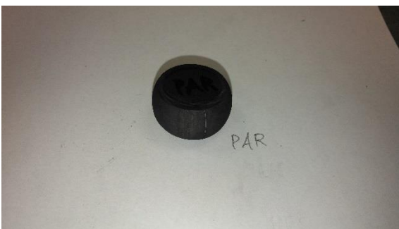
Figure C14. Compression Slug PAR sample after destructive testing. Two hairline fractures were beginning to propagate on the front face of the sample.
