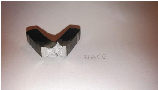
Figure C1. Charpy Impact Base sample after destructive testing. The sample did not completely break, both sides are still connected. Very ductile break.
