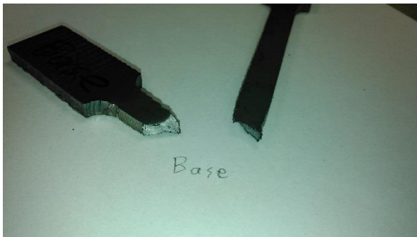
Figure C19. Tension Coupon Base sample after destructive testing.
