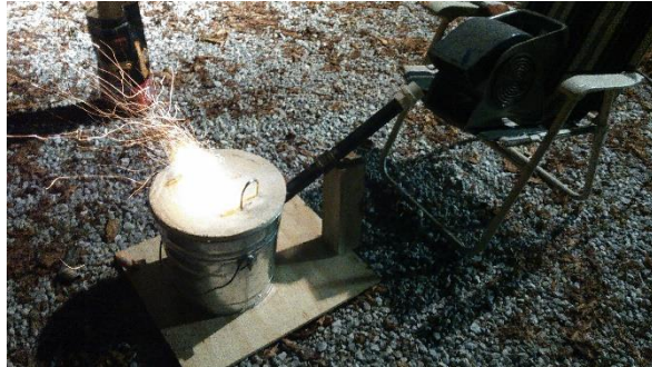
Figure B6. An overall view of the forge with a blower fan during the first test burn.
