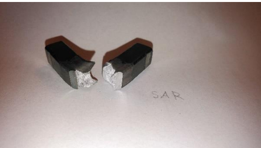
Figure C3. Charpy Impact SAR sample after destructive testing. Ductile break with both sides separating.
