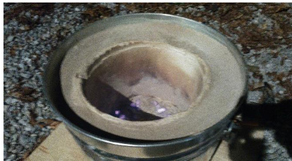
Figure B7. The inside of the forge after the first test burn.
