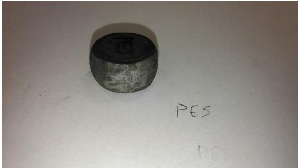
Figure C17. Compression Slug PES sample after destructive testing. Very ductile. No noticeable cracks on the exterior surface of the sample.
