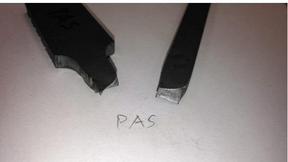
Figure C22. Tension Coupon PAS sample after destructive testing.
