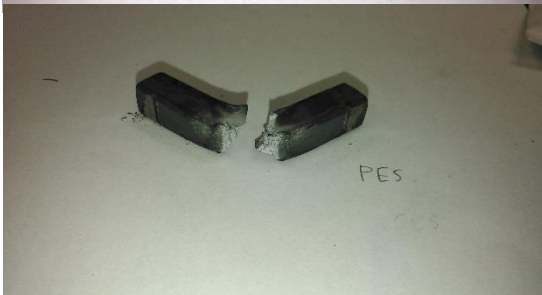
Figure C8. Charpy Impact PES sample after destructive testing. Ductile break with both sides separating.
