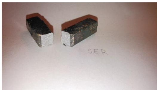
Figure C5. Charpy Impact SER sample after destructive testing. Nearly a perfect shear break. Shows signs of extreme brittleness.
