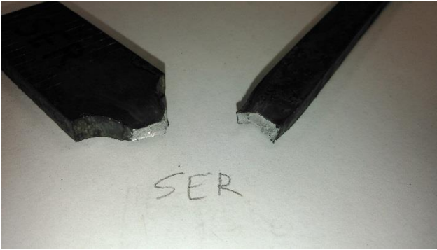
Figure C25. Tension Coupon SER sample after destructive testing.
