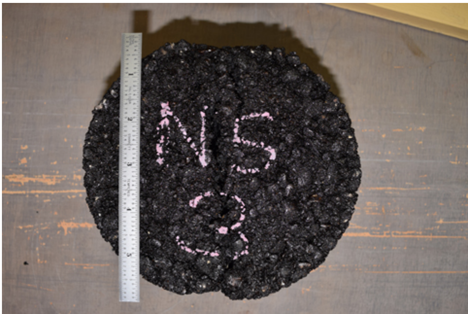
Figure 3b. Example of through-going tensile fracture in NAC cylinder (NS3, 20°C).
