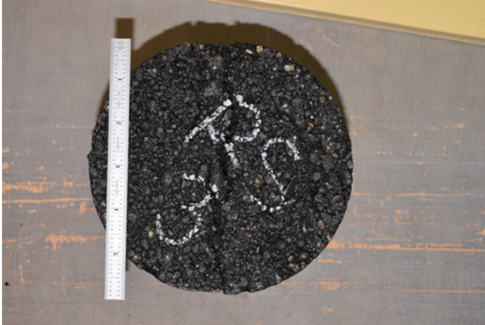
Figure 3a. Example of through-going tensile fracture in RAC cylinder (RS3, 20°C).
