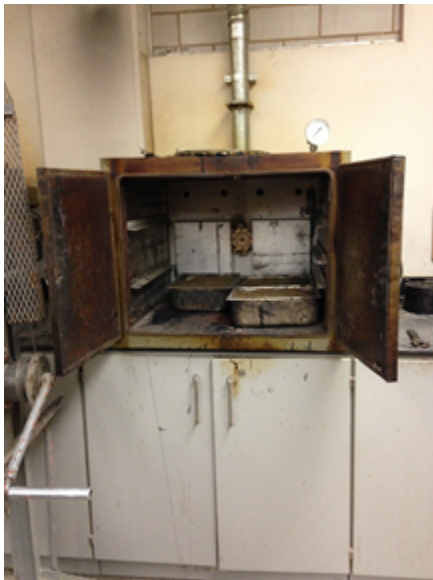
Figure 2: Shown above is the Humboldt MFG. Co. laboratory bench used to dry aggregate sieve size #50.
