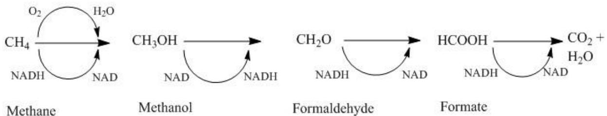
Scheme 1: Methane oxidation cycle used by methanotrophic bacteria.
