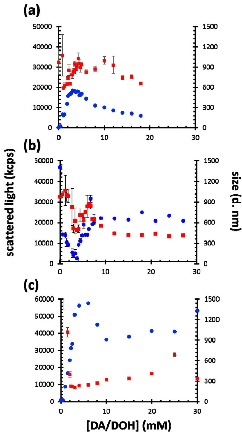
Figure 6. Effect of siderite on the *cvc* of DA/DOH, by light scattering measurements. (a) in the absence of mineral; (b) in the presence of 1 mg/mL siderite; and (c) in the presence of siderite supernatant. Blue circles and red squares correspond to scattered light and size, respectively.
