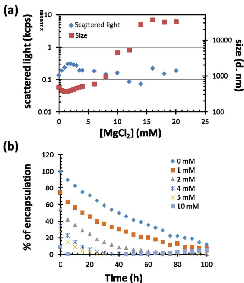
Figure 7. Effect of  $MgCl_2$  on DA/DOH vesicles. (a) Effect of  $MgCl_2$  on the cvc of DA/DOH, determined by DLS. (b) Effect of  $MgCl_2$  on the stability of vesicles, determined by calcein leakage assay.
