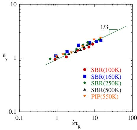
FIG. 3 (color online). The yield strain  $\epsilon_y$  as a function of the applied rate of extension, revealing a master curve with a scaling exponent  $1/3$  for the same five samples after normalizing the strain rate with the Rouse relaxation time  $\tau_R$ .
