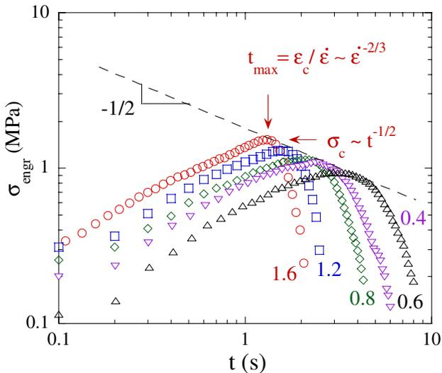
FIG. 1 (color online). The measured tensile force resulting from five discrete continuous uniaxial stretching experiments, expressed in the form of the engineering stress  $\sigma_{\text{engr}}$ , where the numbers 0.4 to 1.6  $\text{s}^{-1}$  indicate the rate of extension. The coordinates of the force maximum (yield point) are designated by  $t_{\text{max}}$  and  $\sigma_y$ .
