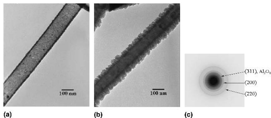
FIG. 8. (a) TEM image of an Al<sub>2</sub>O<sub>3</sub>/Al nanotube prepared by pyrolysis with tube wall thickness of about 10 nm. (b) TEM image of an Al<sub>2</sub>O<sub>3</sub>/Al nanotube with tube wall thickness of about 40 nm. The grain structure of the tube surface is shown. (c) Electron diffraction pattern of nanotubes prepared by pyrolysis.
