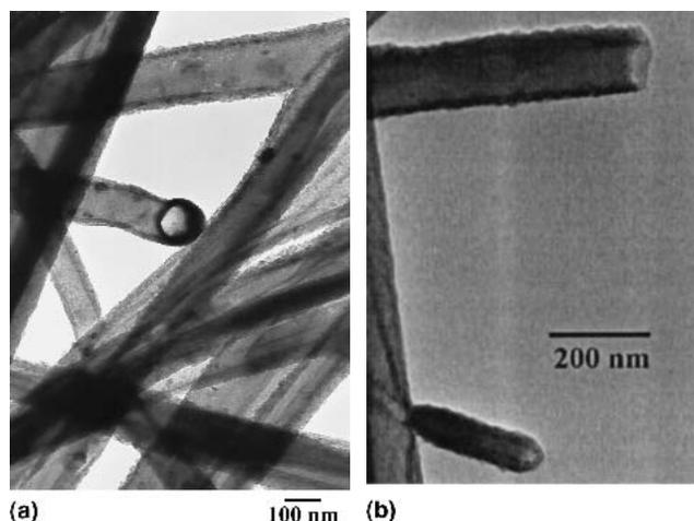
FIG. 7. (a) TEM image of Al<sub>2</sub>O<sub>3</sub>/Al nanotubes prepared by pyrolysis. (b) TEM image of two tube openings. The opening in the smaller tube is about 25 nm.
