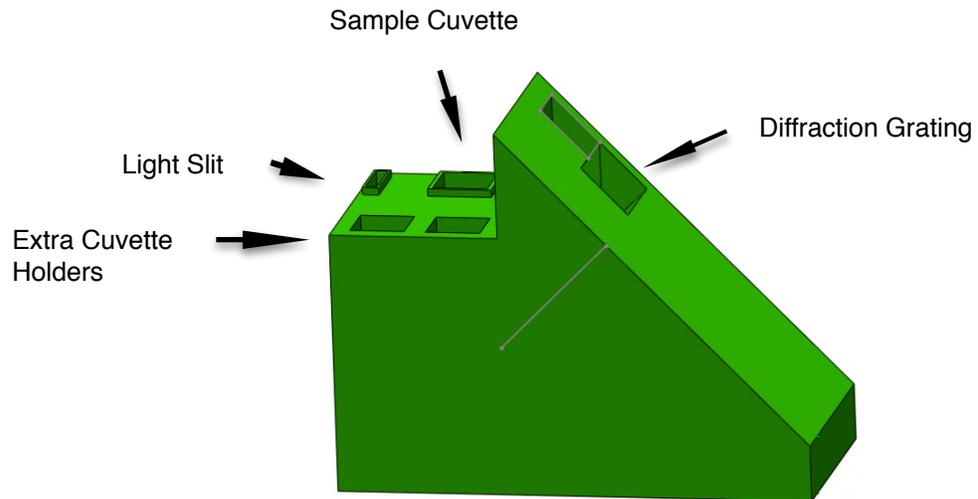
Figure 1: First Version of the Spectrophotometer. The required elements are incorporated without a case for the iPhone to be fixed on the spectrophotometer. The drawing and image was created using SolidWorks version 64, 2014.
