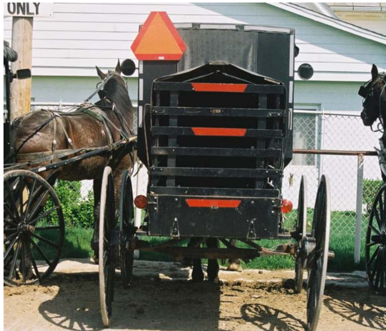
Figure 6: S.M.V. Emblem Mounted on the Upper Left Rear (Ohio)
