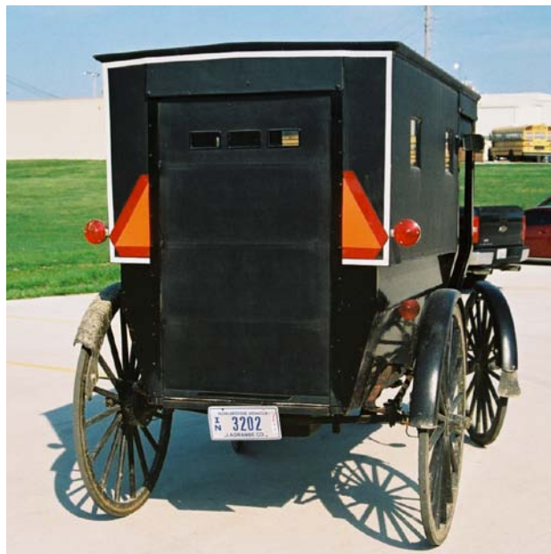
Figure 7: S.M.V. Emblem Split and Mounted on the Rear Sides (Indiana)
