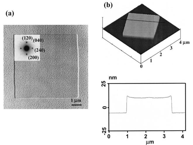
FIG. 2. TEM BF (a) image and AFM height image (b) of a square-shaped “sandwiched” single crystal of the PEO-*b*-PS diblock copolymer crystallized at  $T_x = 25.4^\circ\text{C}$  in chlorobenzene/octane dilute solution. The inset in (a) is an (hk0) SAED of this single crystal with assignments of crystallographic planes. The random PE rod crystals decorated on the surface indicate that the single crystal surface was covered by the amorphous PS blocks.
