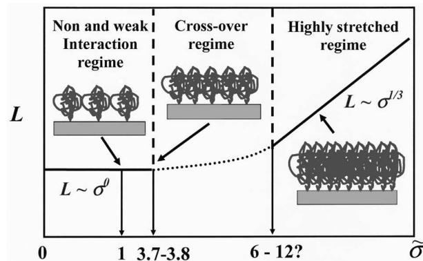
FIG. 1. Schematic representation of the thickness of tethered chains on a substrate in solution versus  $\tilde{\sigma}$ . The  $\tilde{\sigma} = 1$  is the reference point at which tethered chains starts to laterally interact with each other. Note that the tethered chains start to get squeezed by their neighbors at  $\tilde{\sigma}^* \sim 3.7$ – $3.8$  (based on this work).
