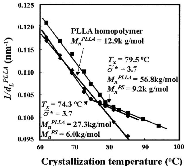
FIG. 4. Relationship between  $(d_L^{PLLA})^{-1}$  and  $T_x$  for the two PLLA-*b*-PS diblock copolymers with different MWs in a good solvent (amyl acetate) can be seen. At  $T_x^* = 79.5^\circ\text{C}$  and  $74.3^\circ\text{C}$ , both of the reduced tethering densities  $\tilde{\sigma}^*$  are 3.7. The  $(d_L^{PLLA})^{-1}$  versus  $T_x$  relationship for a homo-PLLA in the same solvent is also included.
