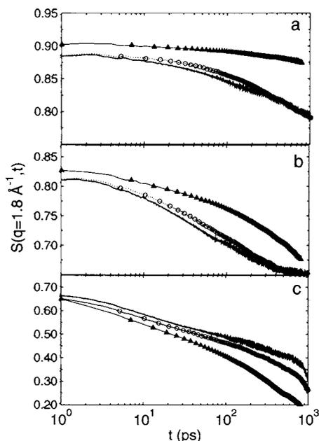
FIG. 6. Incoherent intermediate scattering function for pure trehalose ( $\blacktriangle$ ), and surface ( $\circ$ ) and core (continuous line) hydrogen atoms in lysozyme at (a) 200 K, (b) 300 K, and (c) 400 K.
