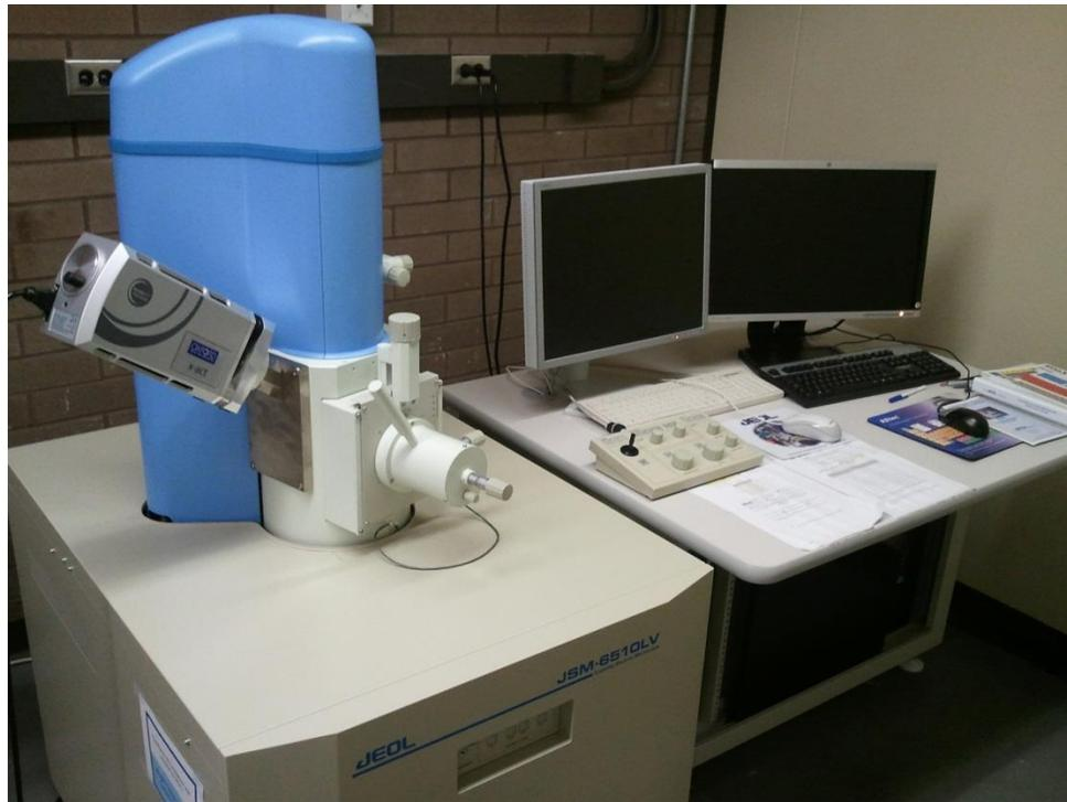
Figure 4.5 Scanning electron microscopy (JEOL JSM-6510LV).
