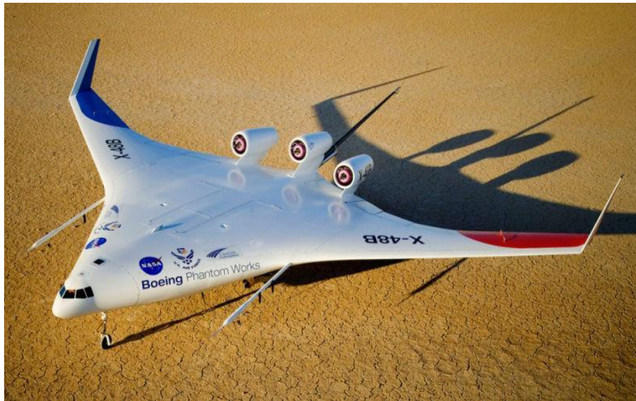
Figure 1: Boeing X-48B: Experimental blended wing aircraft.
