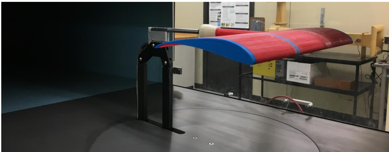
Figure 6: Selig wing mounted in wind tunnel.
