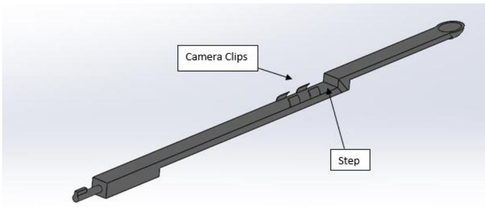
**Figure 11: Attachments with step and camera clips**
