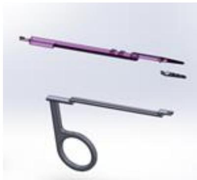
**Figure 9: Exploded view of tweezer attachment**
