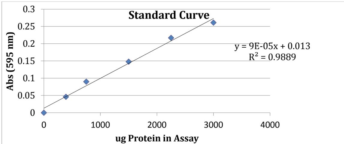
**Figure 5:** Standard curve developed using six standards and the Bradford Assay protocol. Absorbances were recorded at 595 nm, and the linear fit equation generated was used to find the protein concentrations of the four homogenate tissue samples. The  $R^2$  value indicates a relatively linear fit, making it a suitable equation to find protein concentrations of unknown samples.
