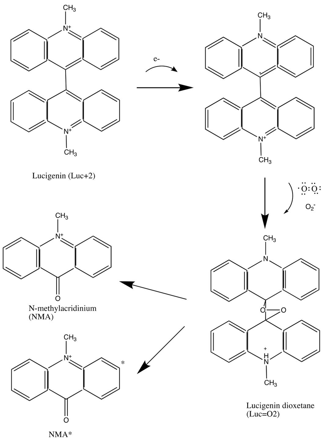
**Figure 3:** Hypothesized reactions undergone in luminometer between lucigenin and a superoxide in order to generate chemiluminescence (Lu, 2006).  $NMA^* = NMA + photon$ . Created using ChemDraw Professional, Version 16.0, PerkinElmer Informatics.
