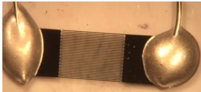
**Figure 4:** Macroscopic view of TOW single-IDT sensor.
