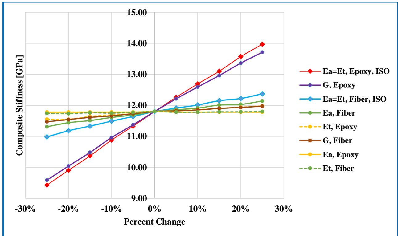
Figure 7: Parametric study of  $[\mp 45]_{2S}$  laminate at room temperature
