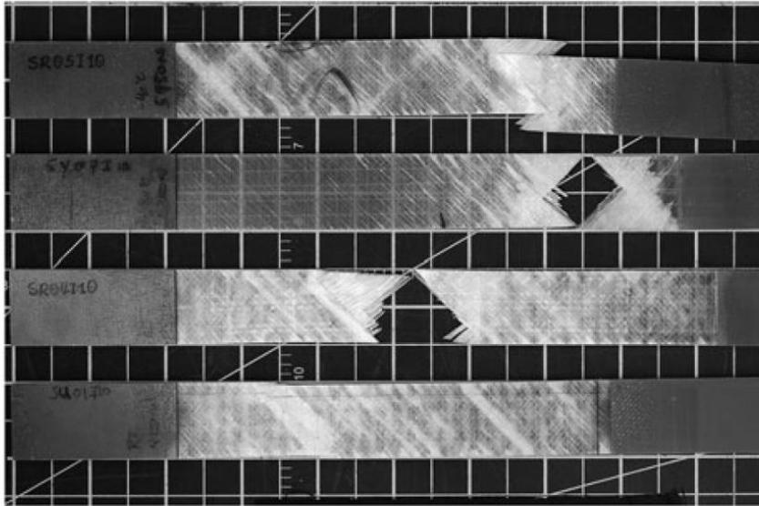
Typical failed  $R = 0.1$  fatigue specimens. From top:  $-40^{\circ}\text{C}$ , 5950 N (86 MPa);  $-40^{\circ}\text{C}$ , 4250 N (63 MPa);  $23^{\circ}\text{C}$ , 5950 N (87 MPa) and  $23^{\circ}\text{C}$ , 4250 N (66 MPa).
