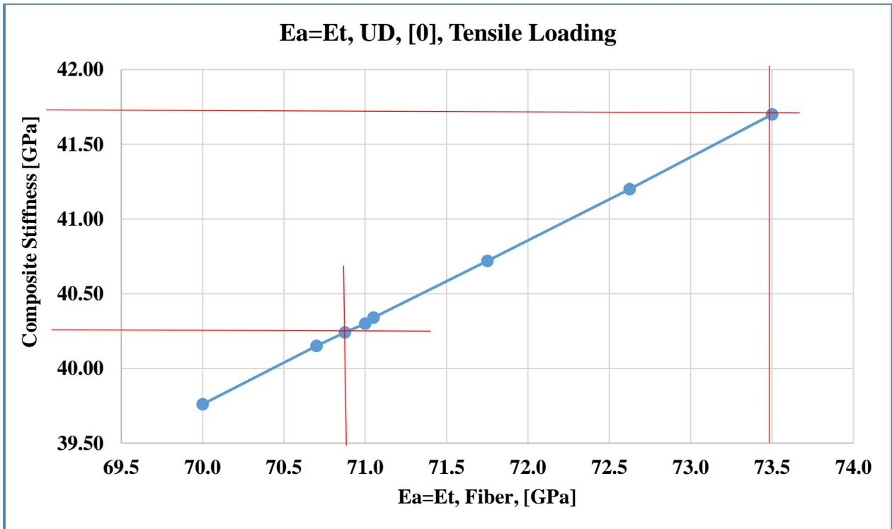
Figure 5: Fiber stiffness prediction at low temperature
