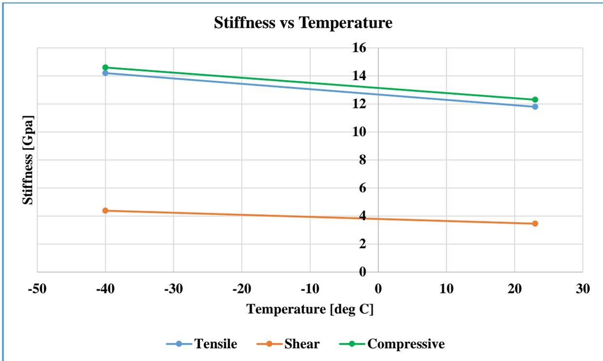
Figure 6: Target composite stiffness values at temperatures of interest
