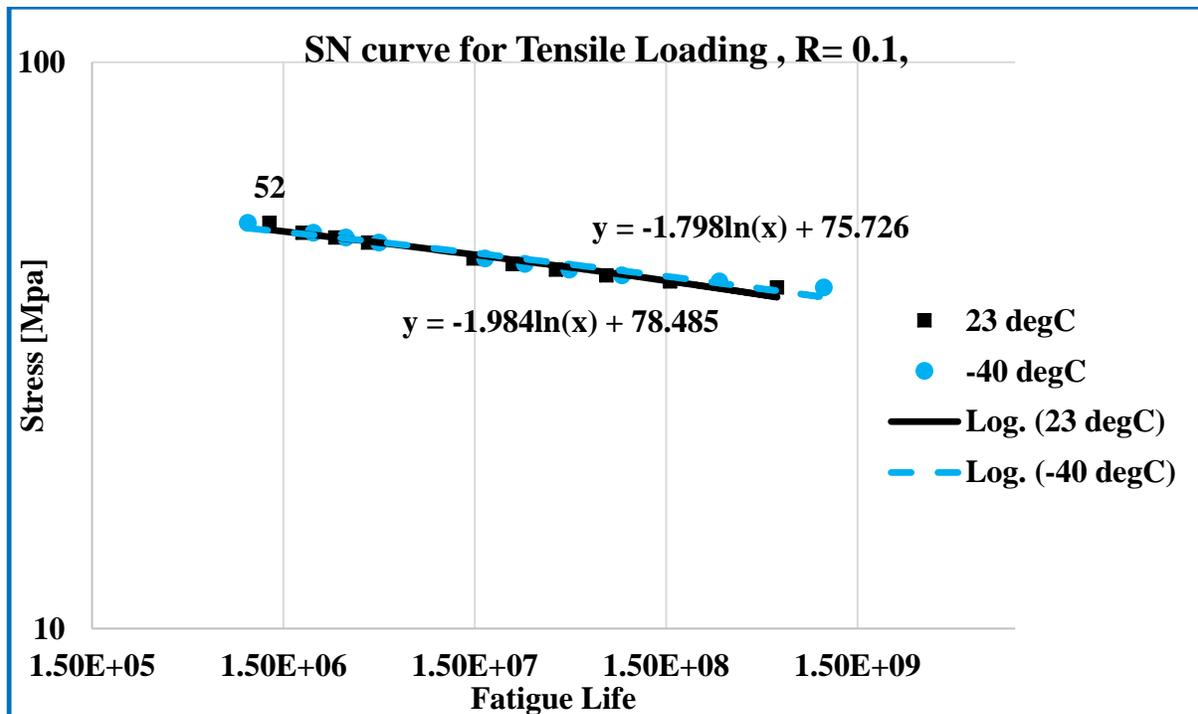
Figure 11: Simulated SN curve of composite under tensile loading
