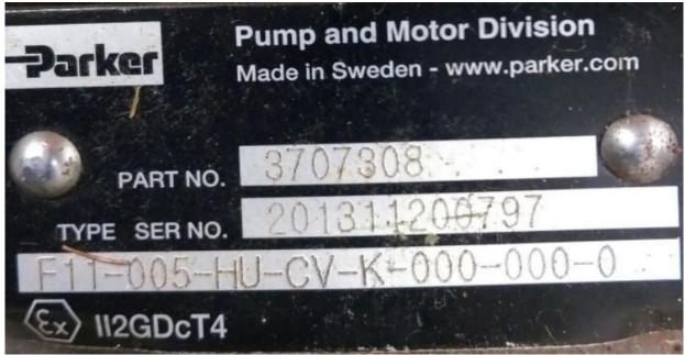
Figure 1: Pump/Motor Part Number
