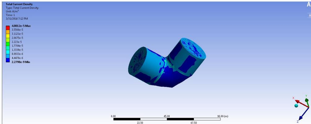
**Figure 5:** Leg-joint model simulated by 10V at joint. Multiple layers of materials are present and able to be customized to fit the isotropic resistivities of human tissue.
