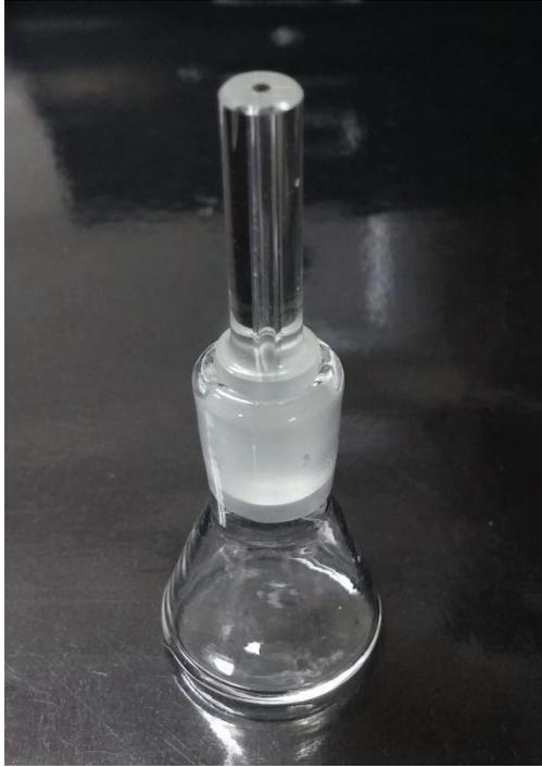
**Figure 4.** The volumetric flask used for density determination of various liquids used in this study.
