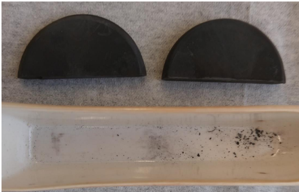
Figure 24 – More spallation products were found near the microcrystalline sample (right) than near the nanocrystalline sample (left)
