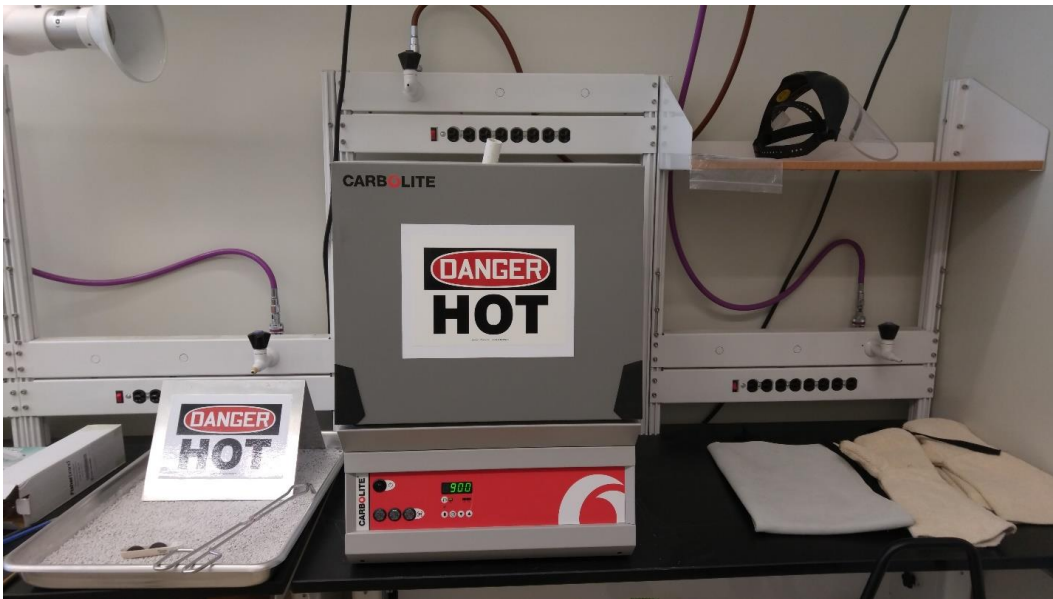
Figure 10 – Experimental setup including hot tray (left), furnace, and PPE (right) including face mask, leather apron, and insulating gloves
