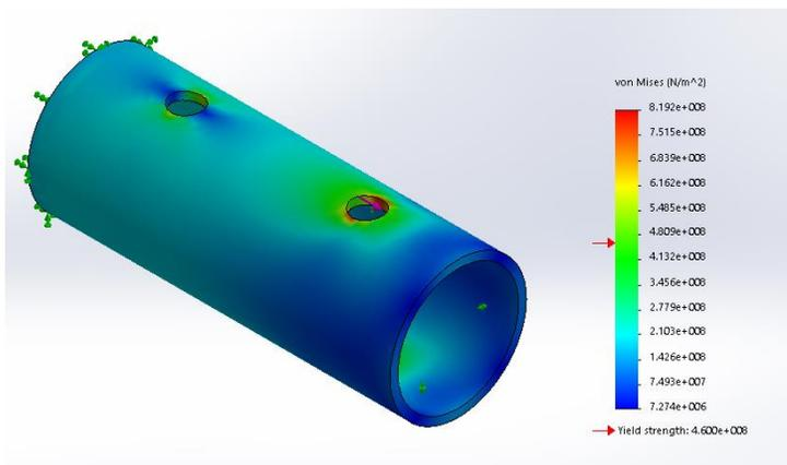
Ultimately, this creates an interesting predicament. There is increased complexity, weight, and manufacturing cost being added to the structure. The titanium, for its weight and high strength looks the most desirable, at least for this test. For manufacturing, having materials of different outer diameters can cause mitering issues. There is also an increase in cost for materials (magnesium and titanium), or post-processing (aluminum). Additionally, the university
