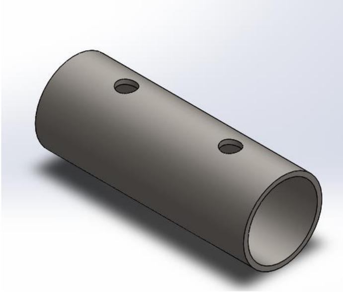
For manufacturing, the double lug section requires welding. No welding is permitted on Titanium and Magnesium alloys. Thus, roughly half of the frame has to be steel or aluminum. Additionally, the 3/16" tabs required are far thicker than other tabs on the car, incurring cost in buying stock, or a weight penalty. For the sleeve, 1.125" x 0.065" wall can be used for 1" OD tubes. Our team uses this material, in limited quantities, for the steering column supports.
