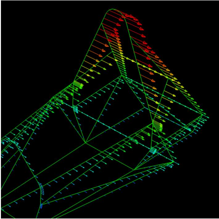
Figure 49: Displacement in Z Direction (Max 0.667")
