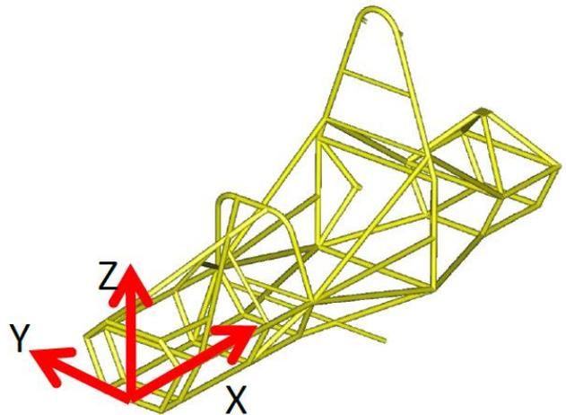
All Simulations require the same boundary conditions, and same failure criteria. The Boundary Conditions are that the nodes at the base of each hoop are fixed against translation in three dimensions, but able to rotate in three dimensions. The maximum allowable deflection is 25 mm, and failure cannot occur anywhere in the structure. Failure is interpreted to mean exceeding the ultimate strength of the member. As a safety factor, my goal is to keep the stress under yield stress.
