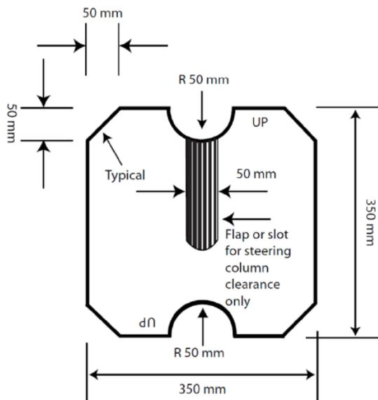
In considering these first two requirements, a multitude of design options become available. The first specifies the shape, and the second the size. It is fully permissible to have a single member be the upper bulkhead support and the front hoop brace. The lower member that defines the floor will serve as the lower bulkhead support. The question is then, how to efficiently add the minimum number of tubes to accommodate suspension points and create good triangulation.
