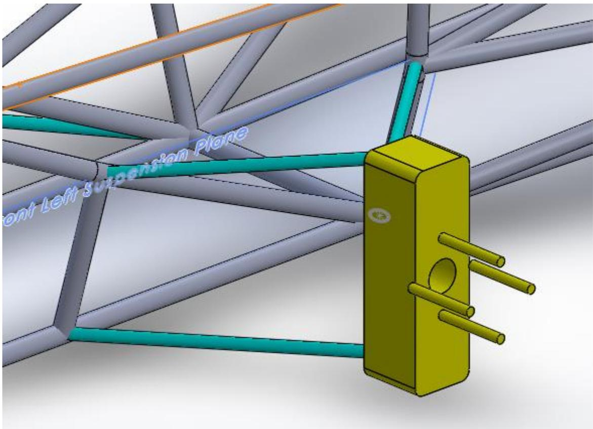
For the rear suspension, the plane is defined at the base of the main hoop, lower bend in the main hoop, and the bottom of the rear bulkhead. The top of the rear bulkhead then is made to
