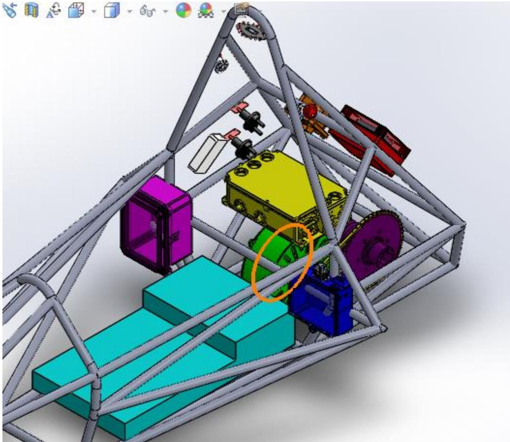
With this, the 95% man can be placed into the car, and the height of the main hoop adjusted to make the frame rules compliant. The positioning of the template also allows for additional Accumulator parts to be placed under his lower back.
