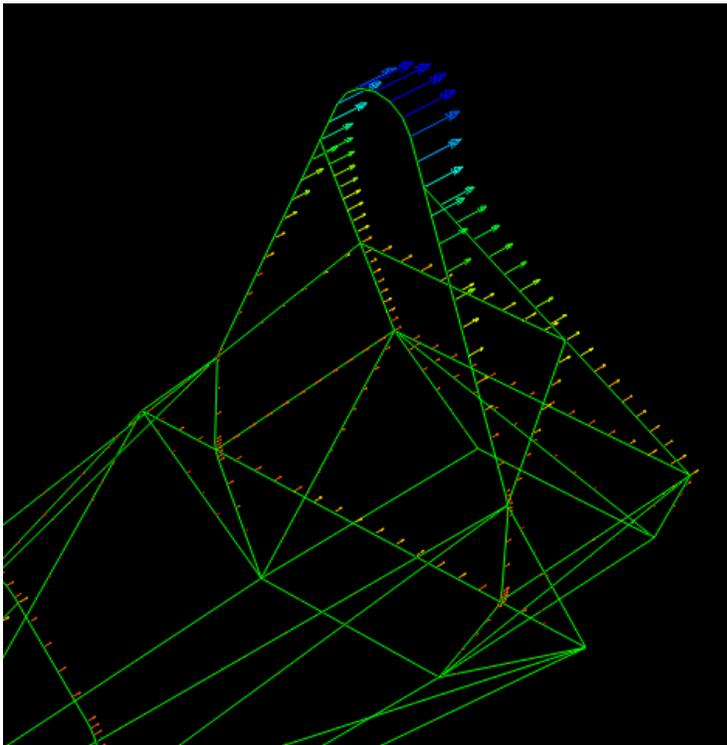
This presents an interesting conundrum. In consulting the micro-iterations done on the rear geometry, raising or lowering the main hoop braces should provide added stiffness. However, in consulting Figures 48, there needs to be stiffness added in the main hoop plane. Using an idea from SAE Baja, the main hoop spar was rotated. The results can be seen in Table 22 Below. Because of the asymmetry, it was tested with the lateral portion of the load applied in both directions
