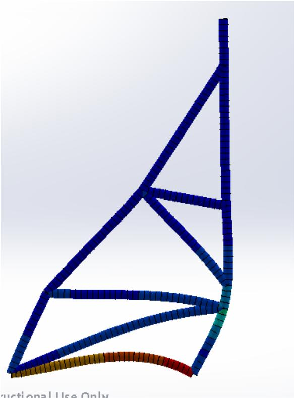
Having obtained a baseline for comparison, 12 alternatives were tested. The alternate designs can be seen in the Appendix. The results can be seen in Table 7. Yield strength of the material is 434 MPa, and the ultimate strength is 668 MPa.
