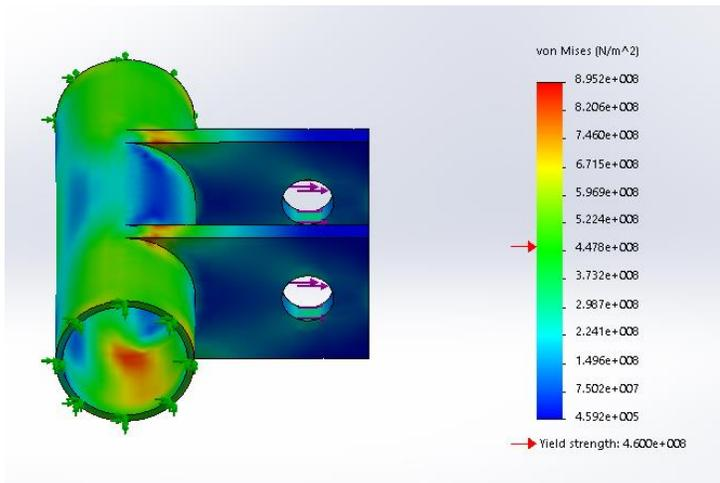
Figure 8: Sleeve Joint at 30KN
