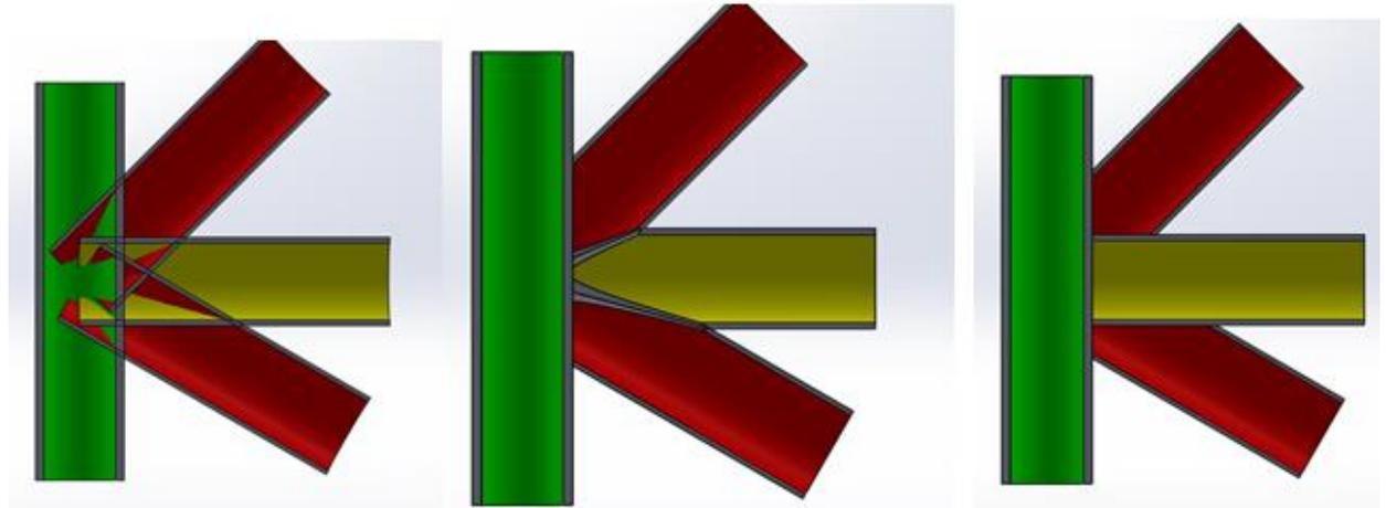
With the part fully mitered, it can be sent out, quoted, and manufactured. For the frame alone on the 2016 car, the cost was approximately \$2660. For the optimized frame, it is \$2250, a savings of \$410 dollars. These figures don't include FSAE student discounts
