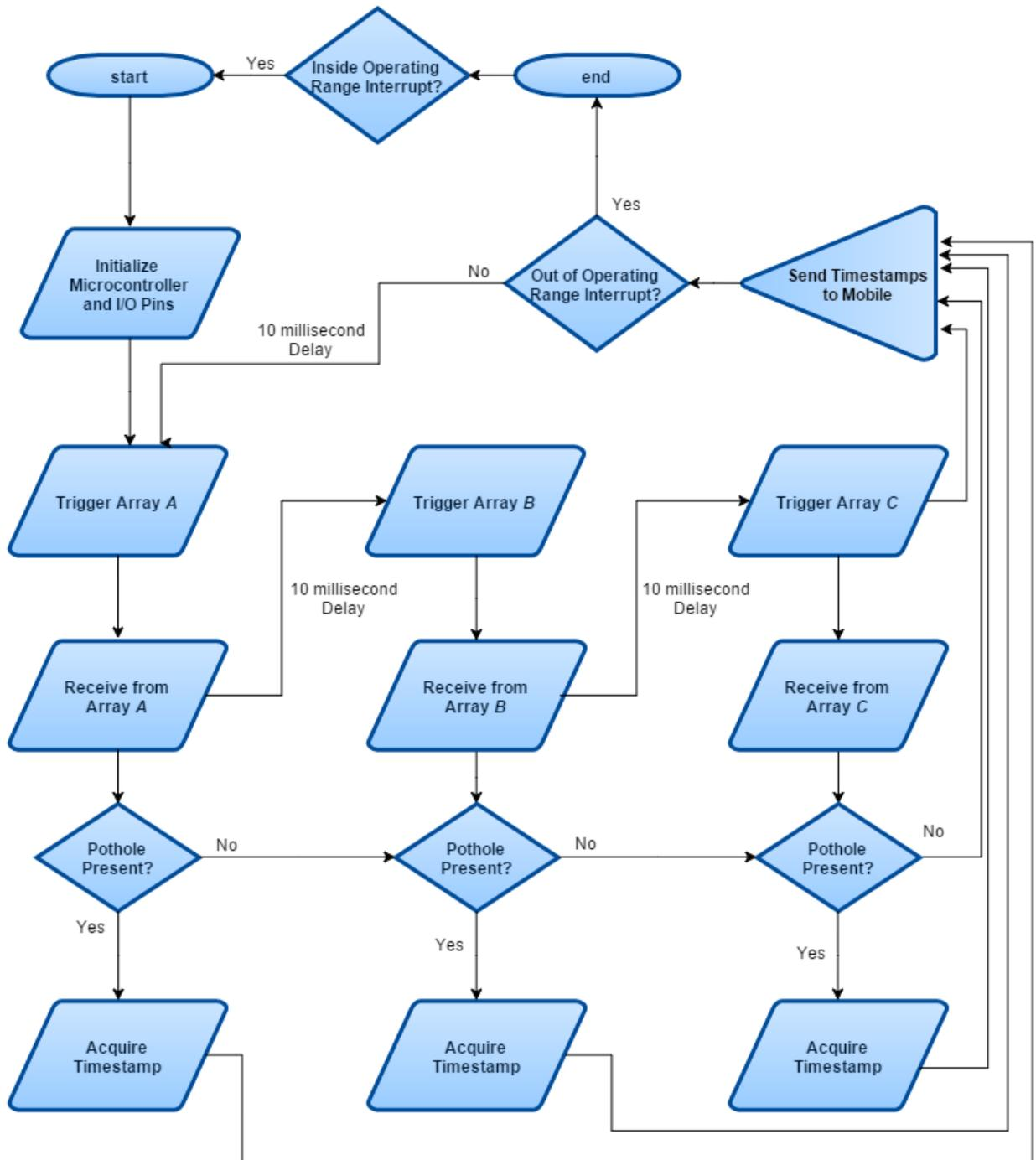
**Figure 13: Firmware Flowchart**
