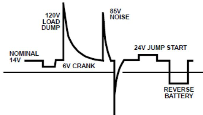
**Figure 2: Test Pulses for Automotive Electrical Systems**
