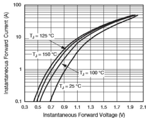
**Figure 4: Forward Voltage Characteristics of Vishay MURS340HE3**
