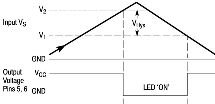
**Figure 5: Input-Output Relation of NCV33161 in Inverting Mode**
