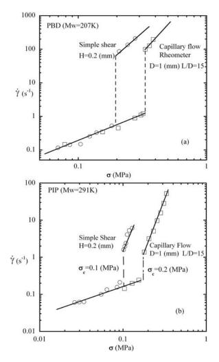
**FIG. 6.** (a) Comparison of 207 K PBD between flow curves obtained with the present CFPSR and the MACR, where the gap *H* is around 0.2 mm and capillary die diameter D=1.0 mm, with the aspect ratio L/D=15 at T=25 °C. (b) Comparison of 291 K PIP between flow curves obtained with the present CFPSR and the MACR, where the gap *H* is around 0.2 mm and capillary die diameter D=1.0 mm, with the aspect ratio L/D=15 at T=25 °C.
