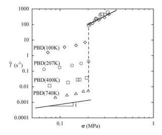
**FIG. 2.** The nominal shear rate, evaluated according to  $\dot{\gamma}=V/H$ , as a function of the applied shear stress for four PBD samples of increasing molecular weight (from  $M_w$ =100 K, 207 K, 410 K to 740 K), where the gap distance *H* is around 0.23 mm at *T*=25 °C.
