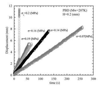
**FIG. 4.** Displacement of the moving inner piston (mm) as a function of time (s) at different stress levels from 0.07 to 0.2 (MPa) for 207 K PBD, where the gap *H* is about 0.2 mm at T=25 °C.
