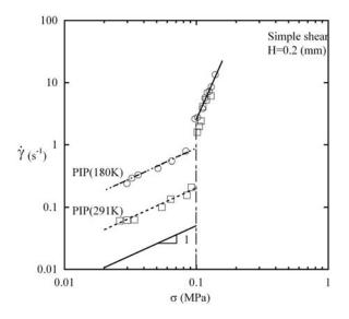
**FIG. 5.** The nominal shear rate, evaluated according to  $\dot{\gamma}=V/H$ , as a function of the applied shear stress for two PIP samples of molecular weights 180 K and 291 K, where the gap distance *H* is around 0.2 mm at T=25 °C.
