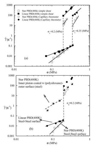
**FIG. 9.** (a) Flow curves of linear and four-arm star PBD at T=25 °C, where the gap is around 0.2 mm in simple shear flow; and in capillary rheometer, the die diameter D=1.0 mm, with the aspect ratio L/D=15. (b) Flow curves of linear and four-arm star PBD with bare and coated inner cylinder surfaces at T=25 °C, where the gap is 0.2 mm.
