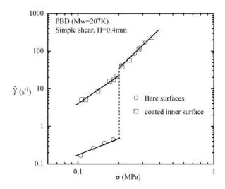
**FIG. 8.** Coating of the inner cylinder wall with a polysiloxane shows the effect of causing wall slip to occur adhesively throughout the applied stress range, leading to the removal of the SST observed with the bare cylinder surfaces. Here, the gap distance *H* is 0.4 mm at T=25 °C. The remaining small jump (in the squares) around 0.2 MPa results from the SST taking place on the outer bare cylinder wall.
