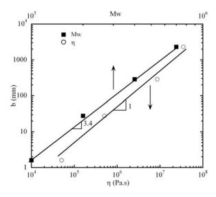
FIG. 3. Extrapolation length b (mm) as a function of the weight average molecular weight  $M_w$  and zero-shear viscosity  $\eta$  at T=25 °C for PBD samples.
