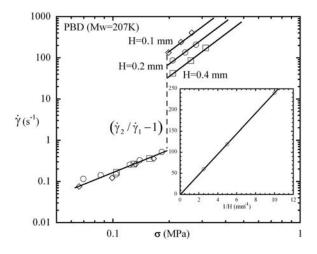
**FIG. 7.** The discontinuous flow transition examined with three different gap sizes as indicated for 207 K PBD at T=25 °C. The inset shows that the abrupt jump in the nominal shear rate as characterized by the ratio  $(\dot{\gamma}_2/\dot{\gamma}_1-1)$  varies linearly with 1/H, in agreement with Eq. (2).
