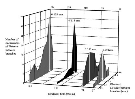
FIG. 3. Distributions of distances between the adjacent branches at different applied electric field (applied potential/gap distance). The distributions are broad at the lower electric fields, so the uncertainties in experimental values are large. The white arrows indicate the most frequently occurring distance between branches at each value of the electric field.
