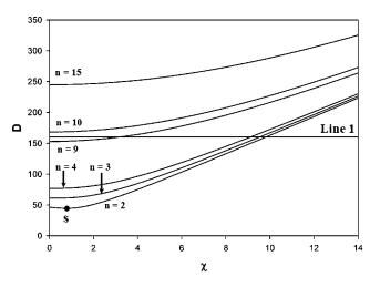
FIG. 6. The straight "line 1" shows the value of D for  $\varphi_0$ =5 kV. The curve n=2 has its lowest value at the point S, which corresponds to the onset of branching. This corresponds to the lowest value of D at which stable undulations can occur. No branching is predicted at lower values of the dimensionless potential D. Also, for the chosen value of  $\varphi_0$ =5 kV, modes with n>9 yield no solutions. Hence, N=9 in this case.
