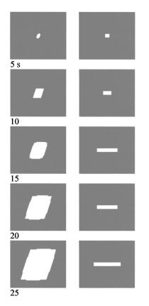
FIG. 10. The spatiotemporal growth of a polyethylene crystal in the crystal order parameter field calculated according to Eq. (21), with the coefficients listed in Table II. The simulated patterns in the first column represent the diamond shaped single crystal in the *x*-*y* plane, whereas those in the second column show the lamellar thickness in the *x*-*z* cross section. The simulations were carried out on a  $64 \times 64 \times 64$  lattice.
