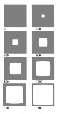
FIG. 2. The emergence of the square single crystal in the crystal order parameter field calculated according to Eq. (7), with  $\tilde{\Gamma} = 0.1894$ , W = 5.086,  $\zeta = 0.256$ , and  $\tilde{\kappa}^2 = 0.1063$  on a 256×256 lattice, showing the temporal increase in the single crystal size.
