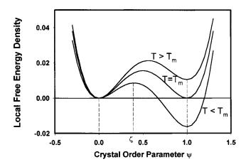
FIG. 1. Schematic plot of the local free energy density and crystal order parameter  $\psi$  for various temperatures showing the metastable energy barrier for a phase transition from the melt ( $\psi = 0$ ) to the crystalline state ( $\psi = 1$ ) with equilibrium at  $T_m$ .
