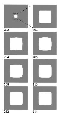
FIG. 3. The enlarged version of the emerging single crystal of Fig. 2, at an interval of 202–214 time steps, exhibiting surface nucleation on four sides (see 204) followed by spreading of the stems along the edges (204–214).
