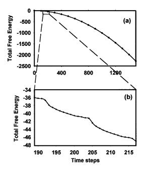
FIG. 5. The free energy dissipation during the course of crystallization showing (a) a monotonous decay over the long time scale corresponding to Fig. 4(a); and (b) a discontinuity in the free energy curve caused by the excess free energy due to successive surface nucleation events taking place on a shorter time span corresponding to Fig. 4(b).
