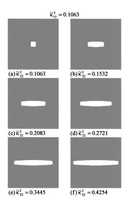
FIG. 6. Various rectangular single crystals calculated based on Eq. (10) using  $\tilde{\Gamma} = 0.1894$ , W = 5.086,  $\zeta = 0.256$ , and  $\tilde{\kappa}_{11}^2 = 0.1063$ , with various values of  $\tilde{\kappa}_{22}^2$ : (a) 0.1063, (b) 0.1532, (c) 0.2083, (d) 0.2721, (e) 0.3445, and (f) 0.4254.
