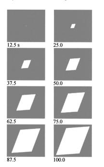
FIG. 9. The spatiotemporal growth of the diamond shaped polyethylene crystal in the crystal order parameter field calculated according to Eq. (11), with the coefficients listed in Table I.
