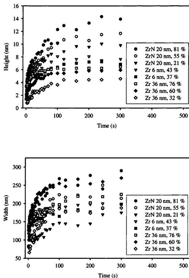
FIG. 2. Time dependence of the oxide-feature height (top) and width (bottom) on Zr and ZrN films. The applied voltage is 8 V and relative humidity varies from 21% to 81%. The legend also indicates the film thickness in each case.
