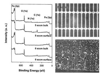
FIG. 3. XPS survey scans of 80-nm-thick iron films sputtered with 0 and 5 SCCM flow rates of nitrogen. Argon sputtering is performed to obtain spectra of the bulk. Optical images of the corresponding patterns formed by applying 300 V for 30 s are shown on the right.
