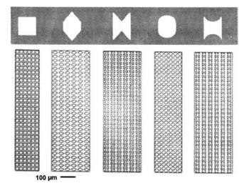
FIG. 1. Optical image of a portion of the silicon stamp consisting of dense arrays of features with synthetic shapes illustrated in the top row. The height of the features is 730 nm.
