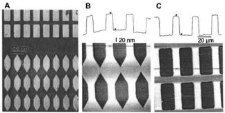
FIG. 4. (A) Optical image of two types of arrays next to each other generated on an 80-nm-thick FeN film. Matching SPM images and cross sections of (B) features with outward triangular and (C) straight end caps are also shown.
