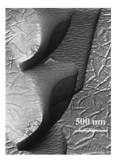
FIG. 6. Low molecular weight PE crystal decorated PET\*-9 flat lamellar crystal and the twisted lamellar crystal observed under TEM. Note that the helical lamellar crystal grows on the top of the flat one. The c axis of the PE crystals (which is perpendicular to the needlelike PE crystals) is parallel to the long axis of both the lamellar crystals. The crystallization conditions are the same as in Figure 2(b).
