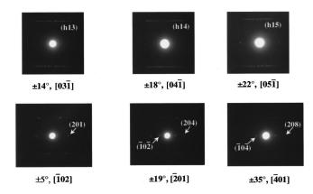
FIG. 4. Set of ED patterns without and with rotations of the  $a^*$ and  $b^*$  axes at different angles obtained from a flat lamellar crystal
