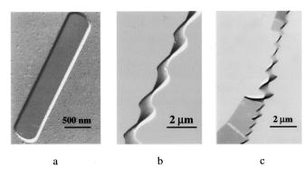
FIG. 2. A flat lamellar crystal grown from the melt at 160 °C for 24 h and observed under TEM (a). A twisted helical lamellar crystal grown from the melt at 145 °C for 24 h and observed under TEM (b). A lamellar crystal grown from the melt at 145 °C for 24 h showing the coexistence of flat and helical crystals, the lower left side showing the microfibers in the crack of the crystal (c).
